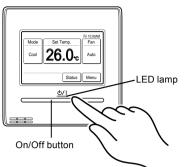
The LED lamp remains lit while the indoor unit is operating.
